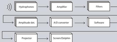
Schematic of simplified system detecting only the signal amplitude
