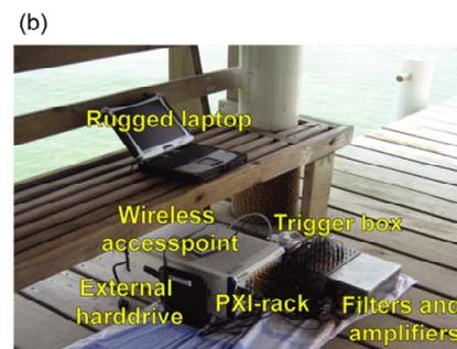
**Figure 3. (a) Basic block diagram of the multi-channel data acquisition system. (b) Photo of the basic parts of the system (hydrophones omitted).**
